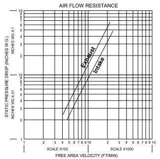
Based on STANDARD AIR- .075 lb. per cubic foot.
