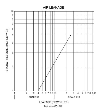
MODEL CFL-D-6 was tested for air leakage in an independent laboratory in accordance with AMCA 500-L
